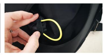
**6.** Cut the new cable in order to have exactly the same length. (The spare cable is black (ref MPPM017). We keep the yellow cable to make picture more understandable.).
